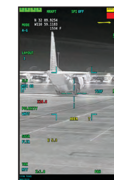
Sensor Control and Display Interfaced for both targeting pods and gimbaled EO/IR devices
